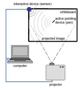
Picture 1. Working principle of an interactive whiteboard
